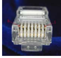
The pin order of RJ-45 crystal head
