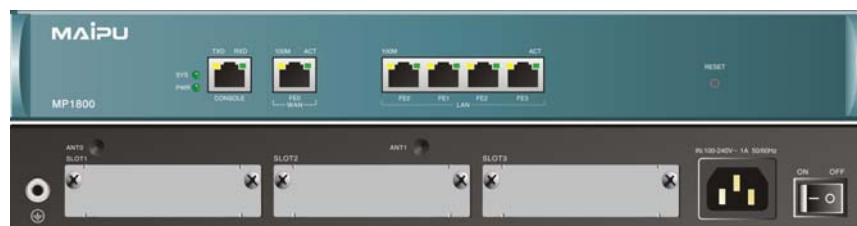
Front and back panels of RM1800-21-AC router
