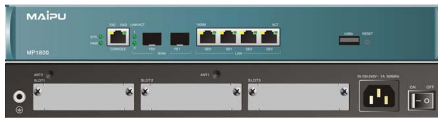
Front and back panels of RM1800-36-AC router
