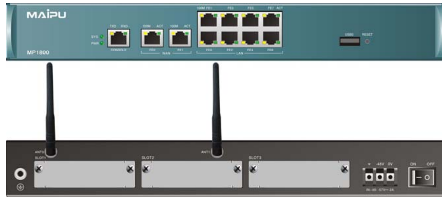
Front and back panels of RM1800-31W-DC48 router
